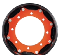
Hub Adapter MSPN 47462 CAI 481115 12 mm thick 1015 carbon steel / reversible 9.0" (228.6 mm) center dia. 8 x 10.75" bolt pattern 0.67" (17 mm) bolt holes, tapered Fits some Bobcat machines
