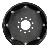
Hub Adapter MSPN 04630 CAI 336820 12 mm thick 1015 carbon steel / reversible 3.68" (93.5 mm) center dia. 10 x 140 mm bolt pattern 0.63" (16 mm) bolt holes, tapered Fits some truck mounted forklifts
