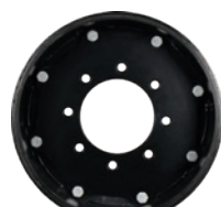
Hub Adapter MSPN 47868 CAI 291074 12 mm thick 1015 carbon steel / reversible 6.0" (152.4 mm) center dia. 8 x 8.0" bolt pattern 0.67" (17 mm) bolt holes, tapered Use adapter to change offset on 8 x 8.0" standard fitment size
