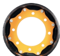
Hub Adapter MSPN 47139 CAI 419992 12 mm thick 1015 carbon steel / reversible 8.75" (222.3 mm) center dia. 8 x 10.91" bolt pattern 0.79" (20 mm) bolt holes, no taper Fits front of Case backhoe loader machines
